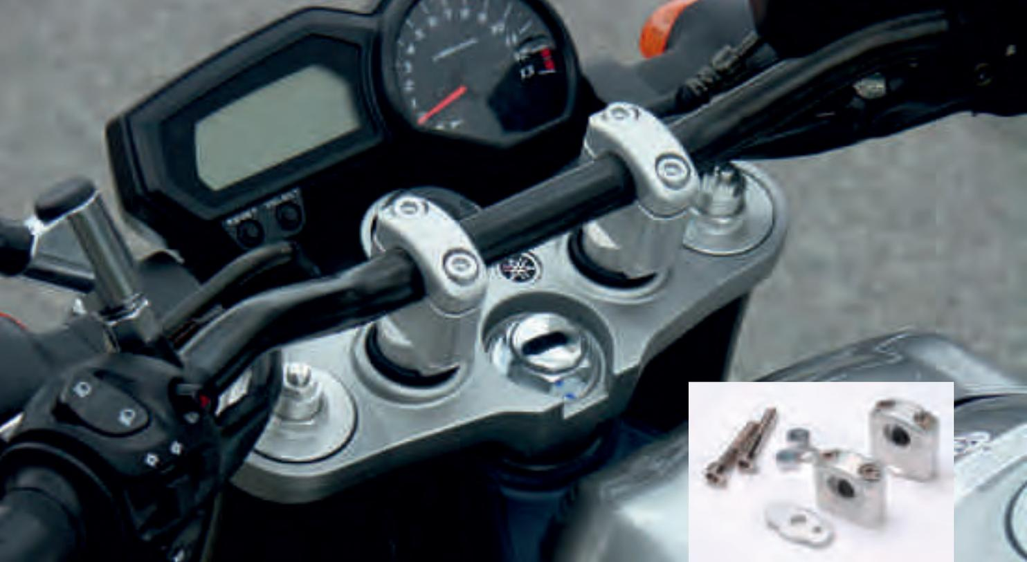
**LSL handlebar clamps** are made for naked bikes with a bolted handlebar mounting. The LSL clamps exchange the original handlebar mounting and bring the bar into a more comfortable position. Depending on the specific model this can be higher, or lower.
