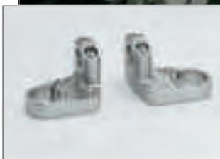
**GL** Top-yoke, CNC-machined, hollowed underside. The original ignition lock can be mounted safely. For modern superbikes, we always use a complete LSL top yoke. To avoid cutting of the fairing tips we use back-set clamps and use a lower and smaller bar "Superbike low" (type N1).
