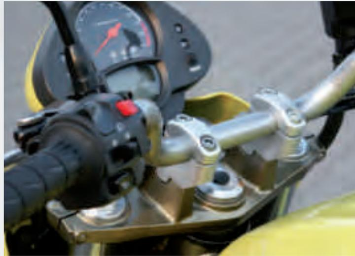
The LSL RiseUp clamps are developed for bikes with standard handlebar clamping. Mounting these clamps on the top yoke raises the handlebar position and brings it closer to the rider. The **RiseUp clamps** are cut out of billet aluminium. Because they are universally designed the clamps fit to almost all 22mm bars. The centre width is 32 to 35mm. The offset backwards is always 16mm; rise is available in 25 and 35mm.
