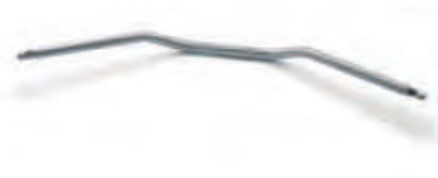
For BMW flat twins with heated grips LSL has developed the bar "M1", which is equipped with welded-in bar ends to carry the original handlebar weights, each 450g. It offers the possibility to feed wires through the 10mm necessary hole in the middle of the bar and is tested for long distance reliability. The bar is made out of steel and matt-silver lacquered.
