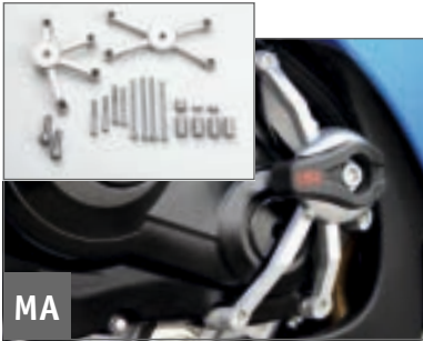
Adapter plate mounted over engine covers.
