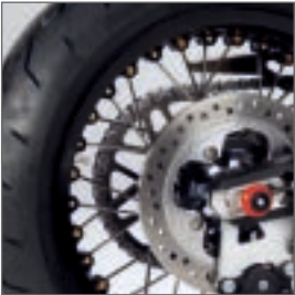
front: 4,4kg incl. Adapter and brake discs rear: 6,9kg incl. Adapter
